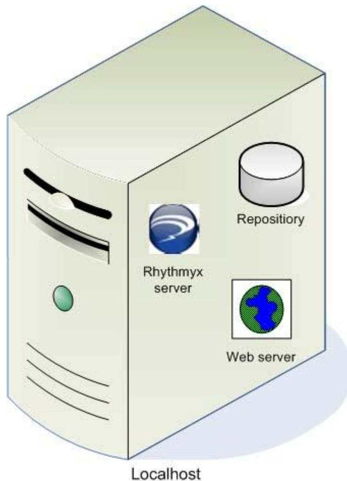
Figure 79: CM System Content Management System with all physical components installed locally
